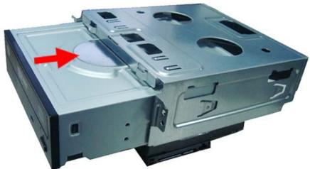
4. Secure the optical drive to the HDD-ODD bracket using two screws.
